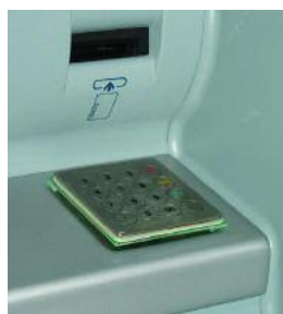
fake PIN pad records PIN entry
