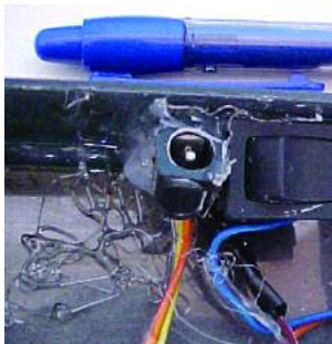
Miniature Video Camera records PIN entry
